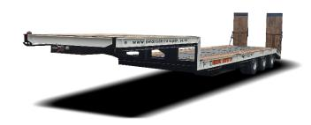
Payload16,000kgLower Deck Height0.9mDeck sizeRefer to chart belowUpper Deck Height1.5mDeck width2.5mTare weight5,750kg
