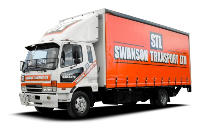
A well-equipped small truck that can carry a moderate payload for its size, with is small size this truck is able to get to small sites and with the tail lift attached this tuck it has the ability to unload itself with the use of a pallet jack.
