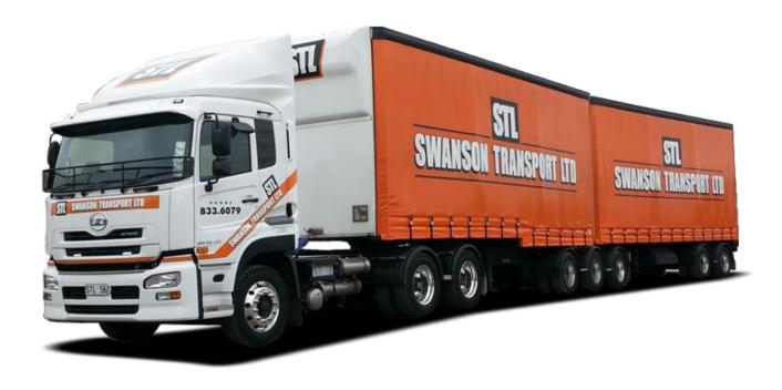
Our B-train can be utilized for bulk movement of stock across Auckland, the 1<sup>st</sup> trailer has a moveable step deck platform to allow pallets to sit on a flat surface and not overhang the step while in transit.
