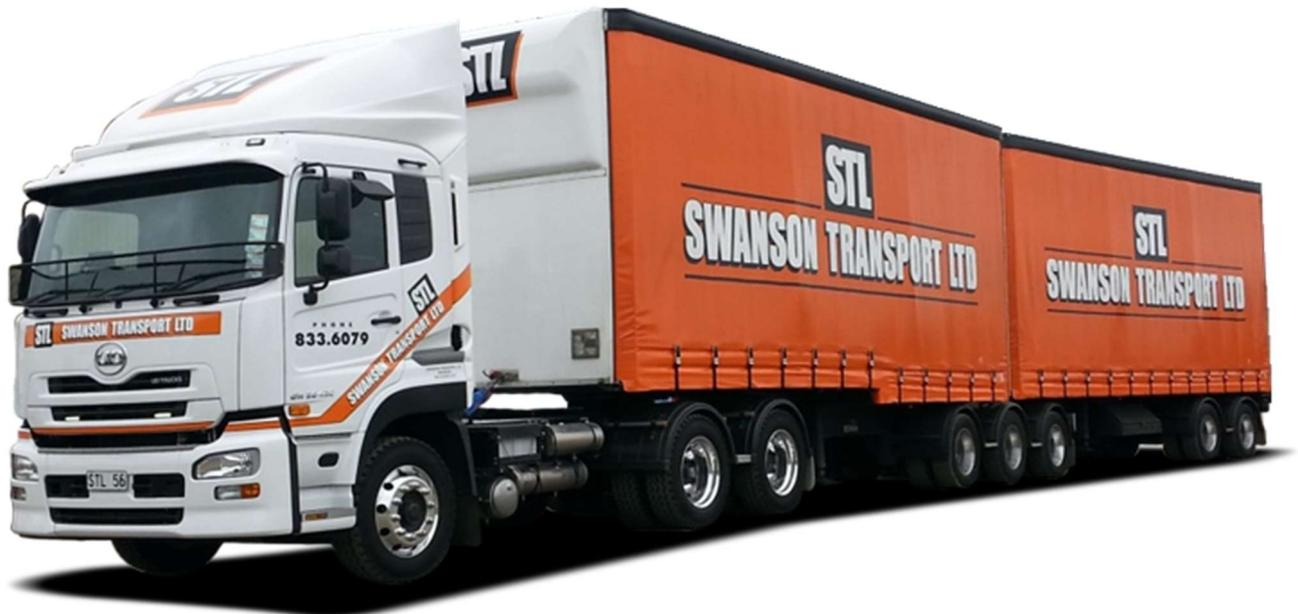
Our B-train can be utilized for bulk movement of stock across Auckland, the 1<sup>st</sup> trailer has a moveable step deck platform to allow pallets to sit on a flat surface and not overhang the step while in transit.
