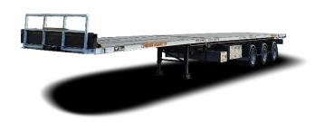
Payload Deck Height 1.3m Refer to chart below Deck size Tare weight 8,300kg
